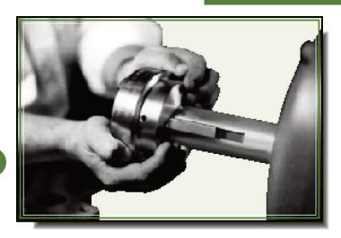
**Shaft spacing** should be within range given by dimensions 'W' and 'X' as shown in charts on page 3.
