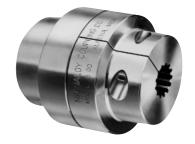
Magnaloy's close machining tolerances (TIR of .002") assures vibration-free operation and easy, accurate alignment without need for special tools. Solid magnesium alloy permanent mold castings are heat treated and offer the highest strength-toweight ratio available.
