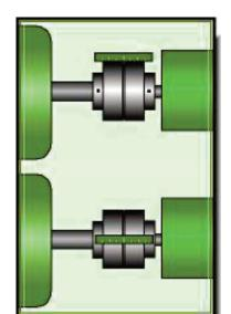
Perfect alignment of equipment shafts, in most cases, is impractical to obtain or maintain, and misaligned equipment produces, excess stress on bearings and the coupling. Magnaloy's insert design will accept misalignment strain and, when excessive, will cause insert wear as a visual and audible indication of misalignment problems. However, Magnaloy's inserts are inexpensive and easily replaces; under normal conditions the insert seldom requires replacement.
