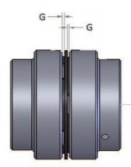
Loose Fit - up to additional gap shown on chart to accommodate motor shaft float
