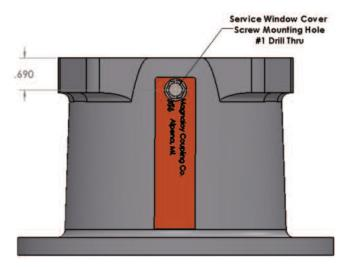
M056 Mount with New Cover installed. The Cover has been cut to length to cover the Service Window Opening. The mount has been drilled at the indicated location and the mounting screw installed.
